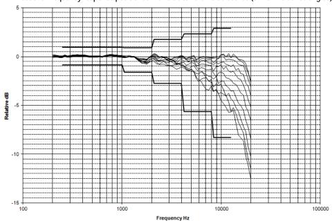
Directional frequency response positioned using side toward noise source (0°-150° incidence angles)
